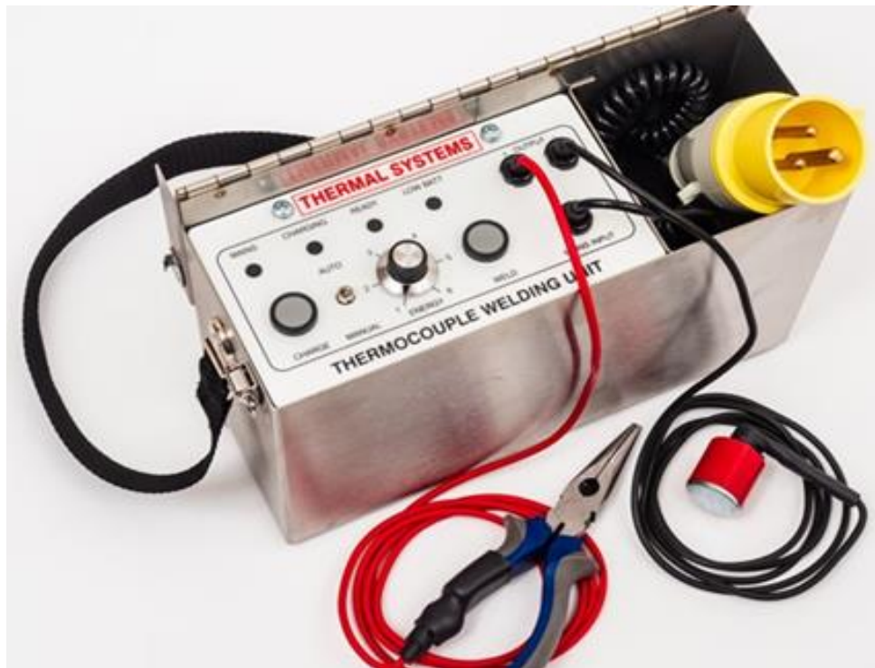
FIGURE 8 – CAPACITIVE-DISCHARGE THERMOCOUPLE ATTACHMENT UNIT (TAU) USED FOR WELDING TYPE K THERMOCOUPLE WIRE DIRECTLY TO COMPONENT SURFACE
